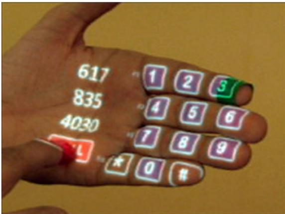
Figure 5.7: Touch detection on projected surface
