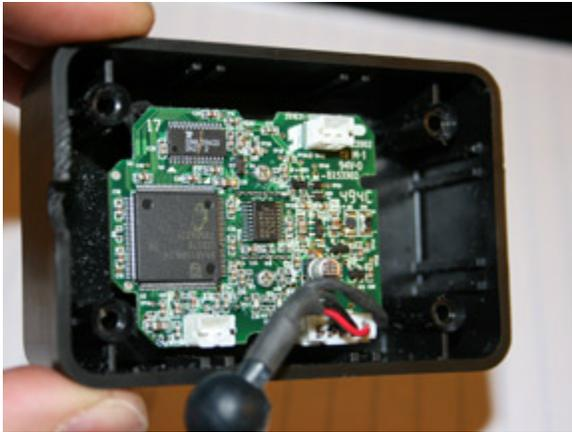
Figure 4.8: Housing for modified camera PCBs
