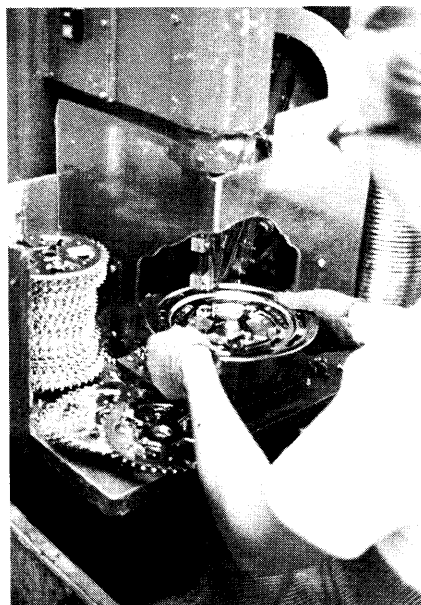
Chain-guard and sprockets are assembled with machine that automatically drives bolts with machine that automatically drives bolts to desired torque. While other in-house production operations will be eliminated by new purchased plastic component, this operation will remain essentially the same.
