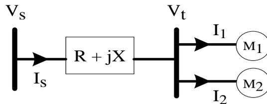
Figure 3.1 Single Line Diagram.
