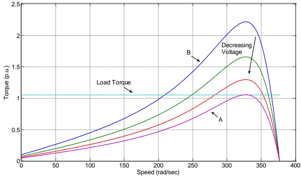
Figure 3.3 Torque (p.u.) - Speed (rad/sec) Curve for Decreasing Voltages.
