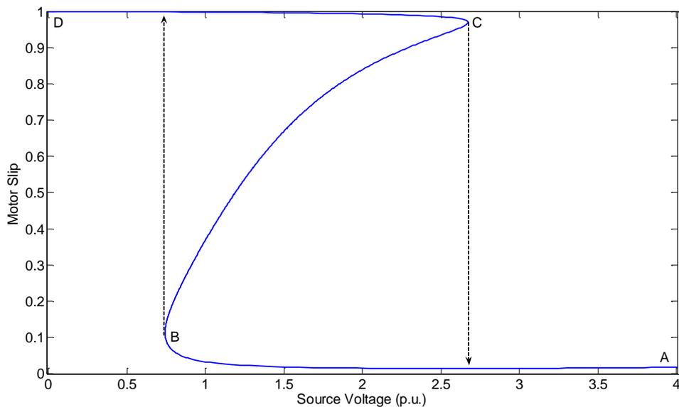
Figure 3.6 Motor Slip vs Source Voltage (p.u.).
