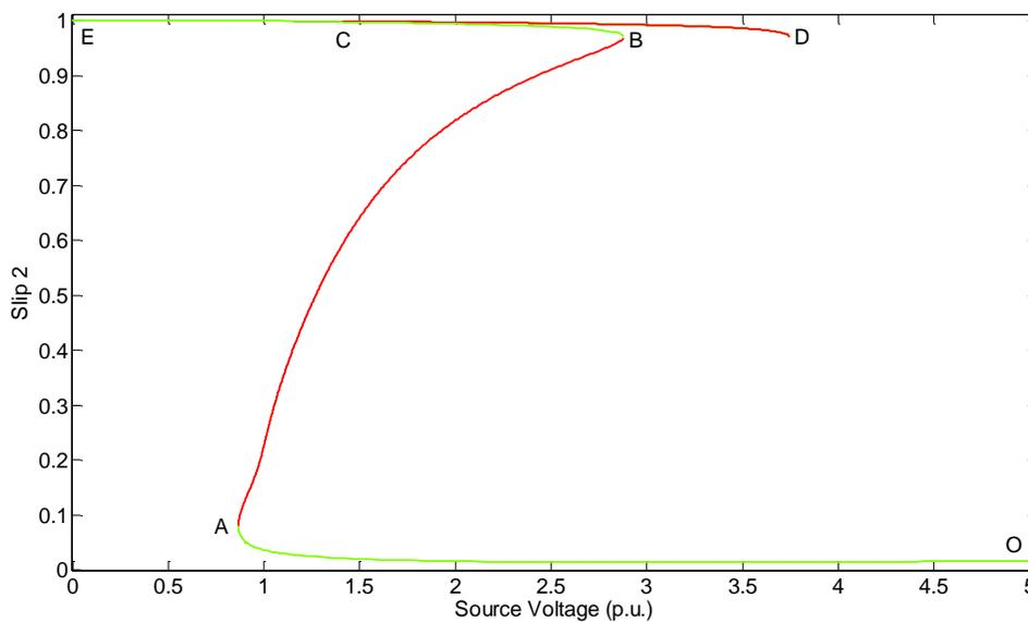
Figure 3.9 Motor 2 Slip vs Source Voltage (p.u.).
