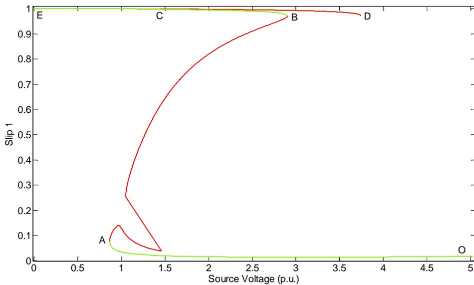
Figure 3.11 Motor 1 Slip vs Source Voltage (p.u.).
