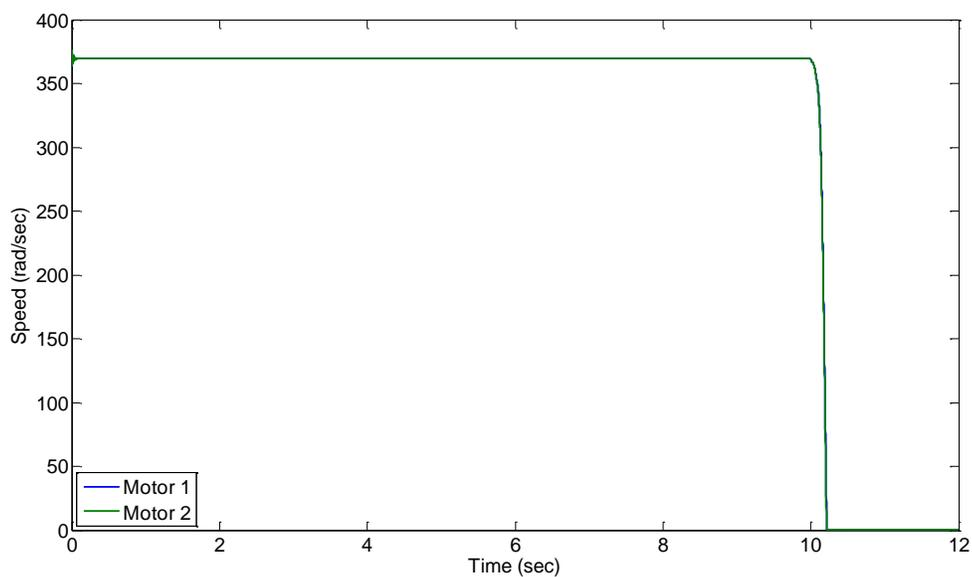
Figure 3.16 Motor Speed (rad/sec) vs time (sec) with both stalled.
