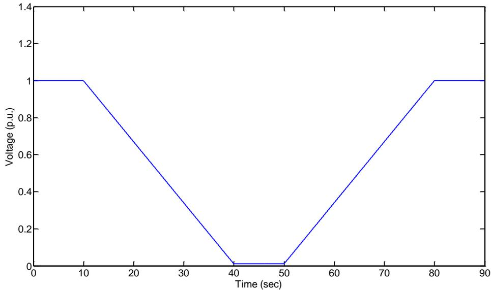
Figure 2.1 Voltage (p.u.) vs Time (sec) for Ramp Test.
