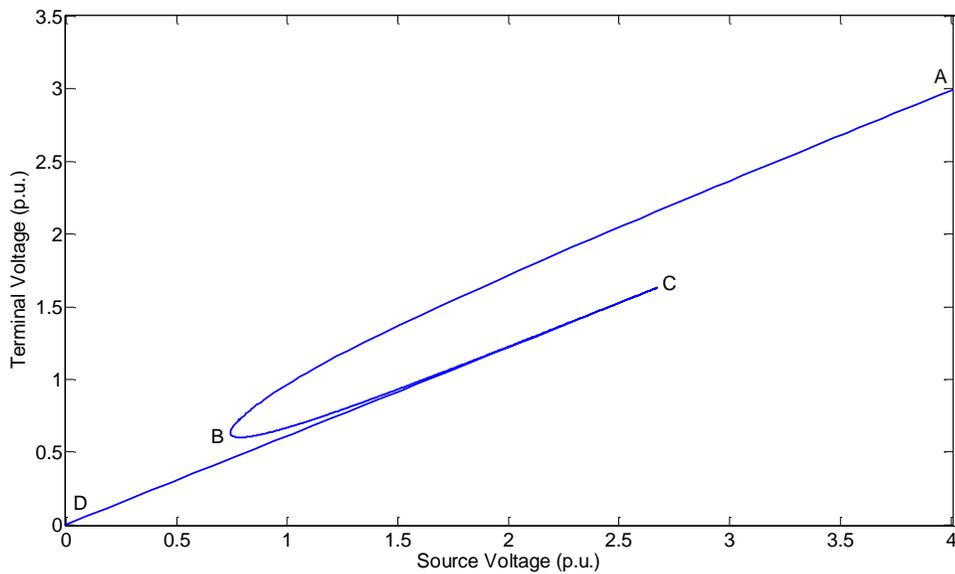
Figure 3.7 Motor Terminal Voltage (p.u.) vs Source Voltage (p.u.).
