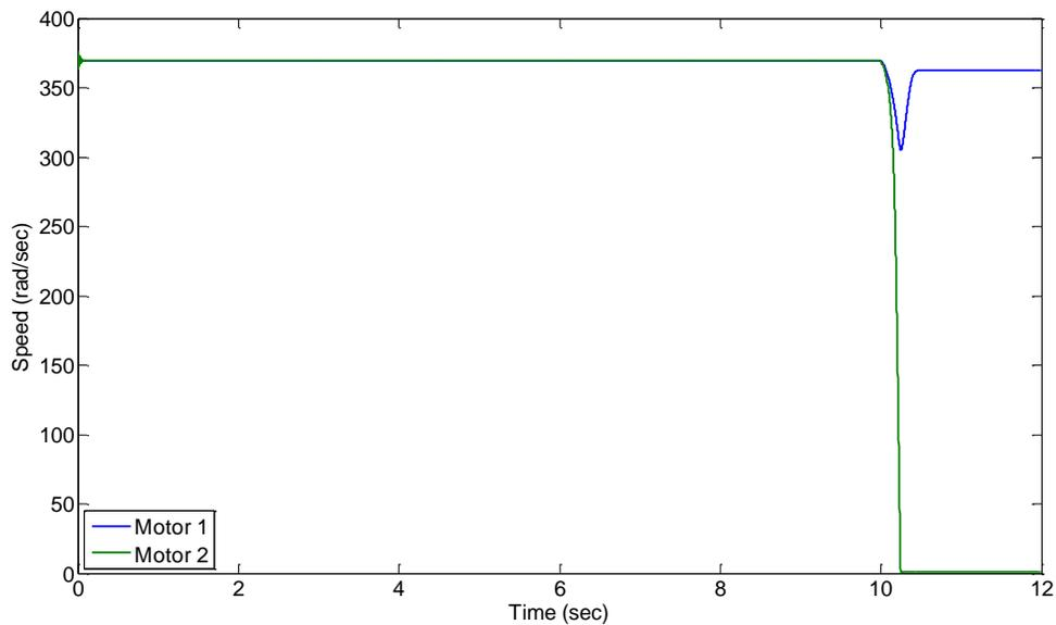
Figure 3.15 Motor Speed (rad/sec) vs time (sec) with one stalled, one running.
