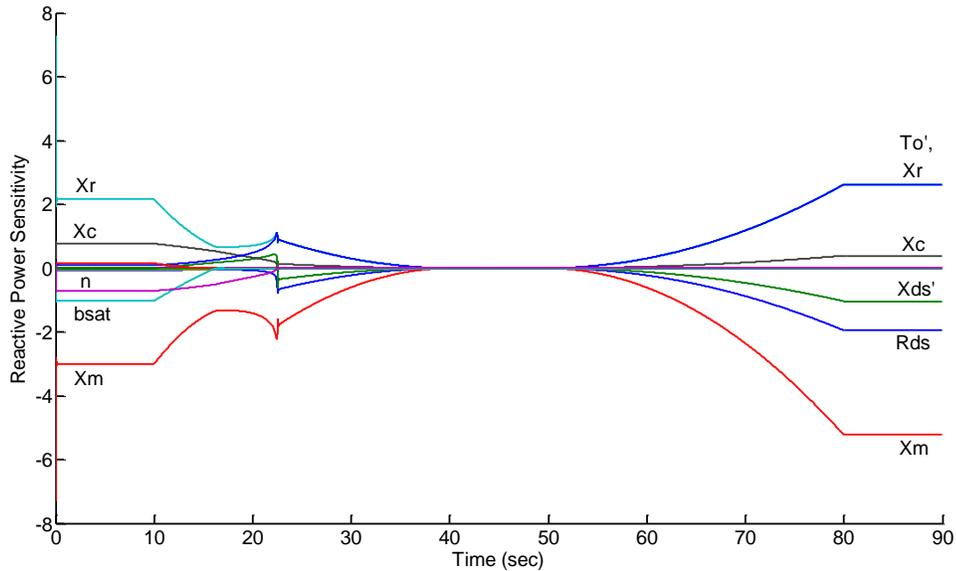
Figure 2.9 Relative Sensitivity of Reactive Power vs Time (sec) for Ramp Test.
