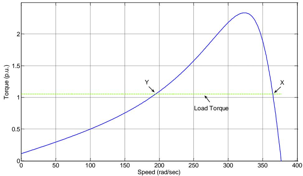
Figure 3.2 Torque (p.u.) - Speed (rad/sec) Curve.
