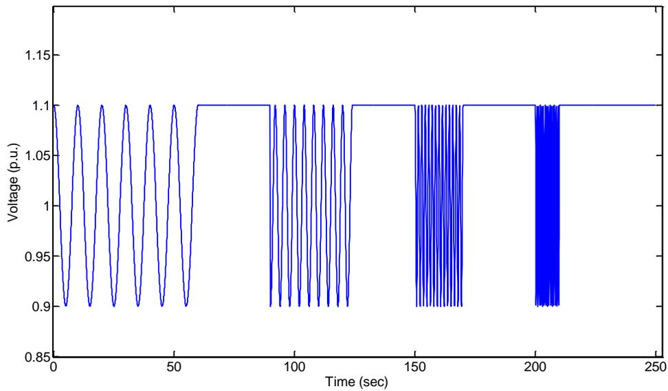
Figure 2.10 Voltage (p.u.) vs Time (sec) for Sinusoidal Test.
