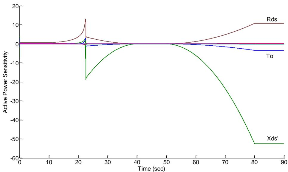
Figure 2.7 Sensitivity of Active Power vs Time (sec) for Ramp Test.
