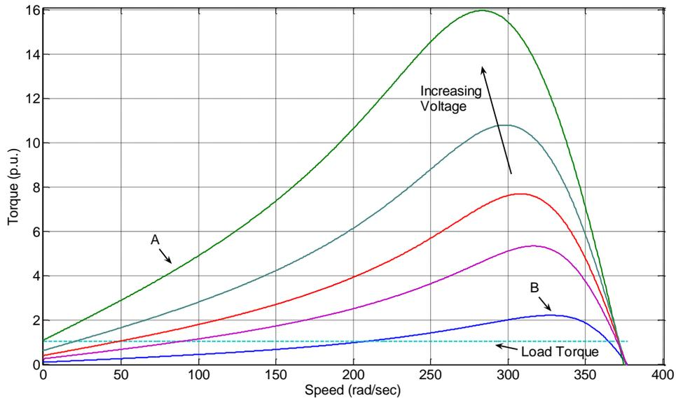
Figure 3.4 Torque (p.u.) - Speed (rad/sec) Curve for Increasing Voltages.
