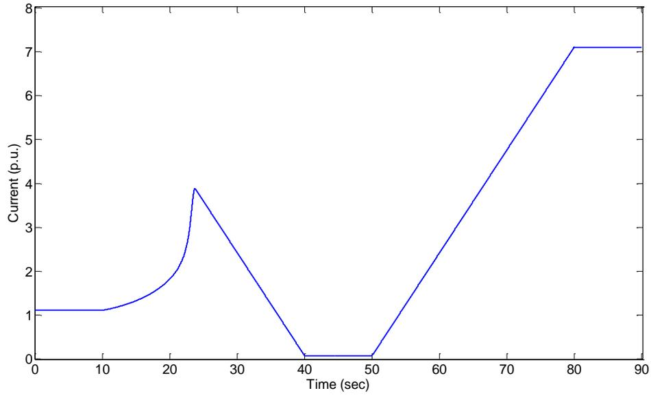
Figure 2.3 Current (p.u.) vs Time (sec) for Ramp Test.
