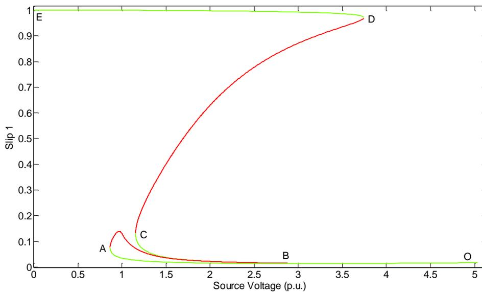
Figure 3.8 Motor 1 Slip vs Source Voltage (p.u.).
