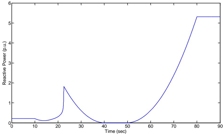
Figure 2.5 Reactive Power (p.u.) vs Time (sec) for Ramp Test.
