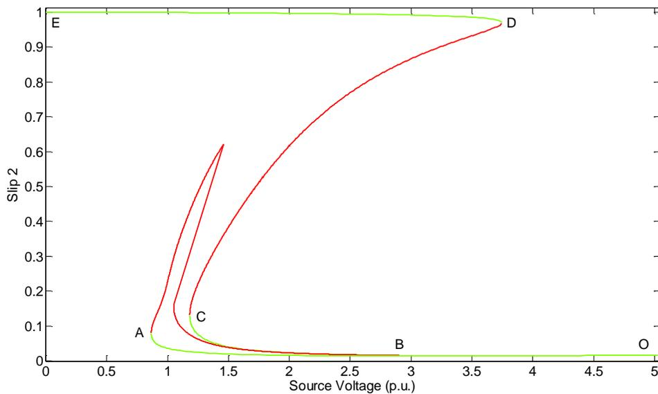
Figure 3.12 Motor 2 Slip vs Source Voltage (p.u.).
