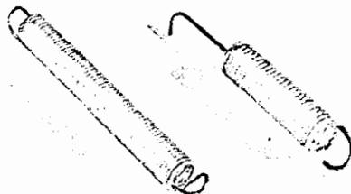
Converting special spring to standard (left) reduced the cost from 9c to 3c.
