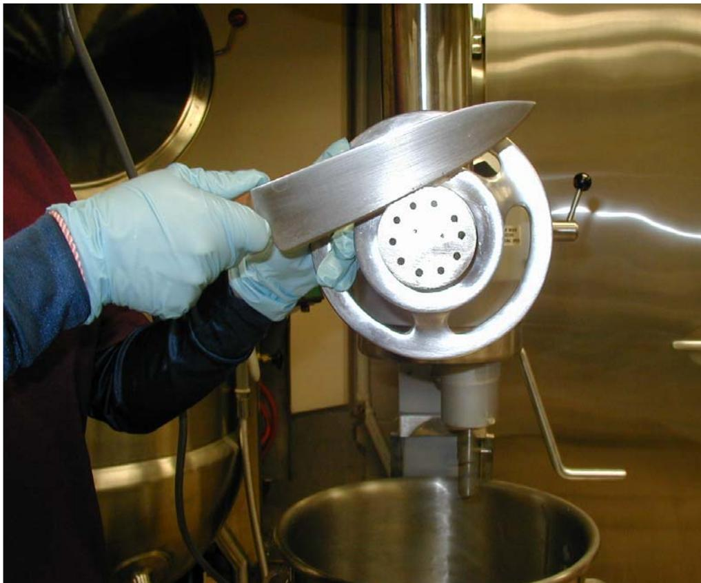
*Figure 9.* Die attached to the Hobart extrusion attachment
