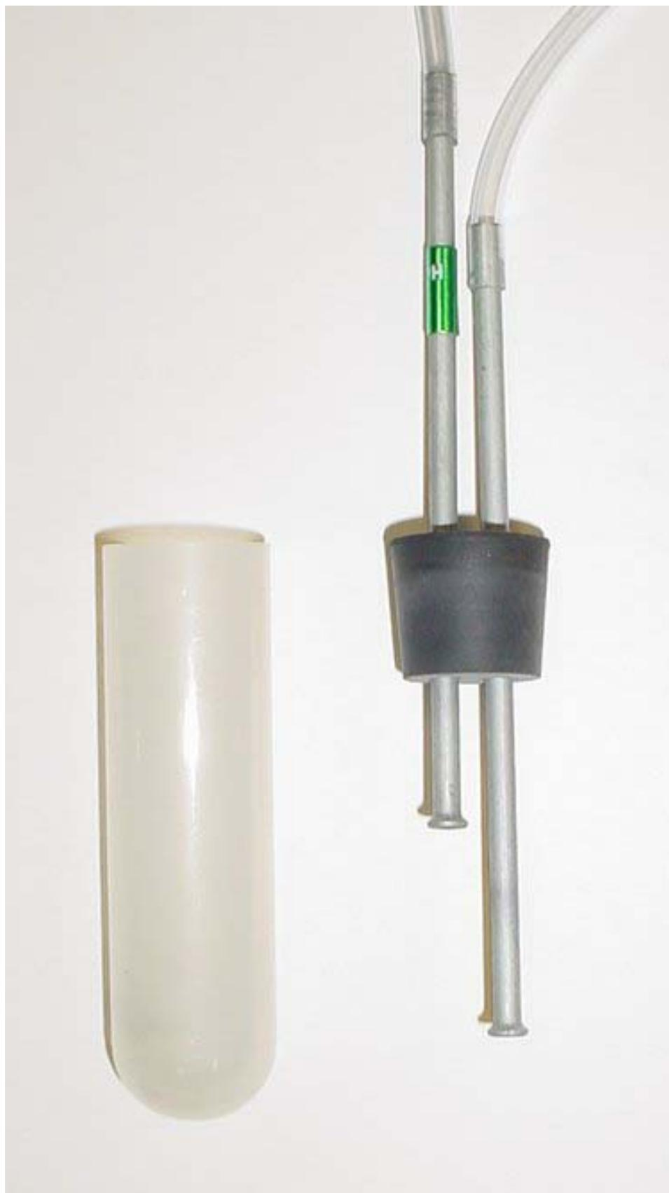
**Close Up Of The Feeder System Test Tube**
