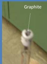
Graphite paint applied to the electrical contact.
