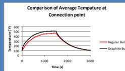
Graph indicates that graphite paint reduces contact temperature.
