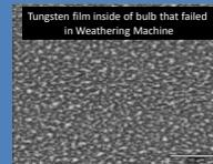
Tungsten film inside of bulb that failed in Weathering Machine
