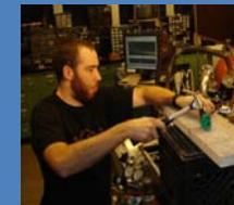
Smashing a halogen light bulb to determine if the halogen gas leaked out.
