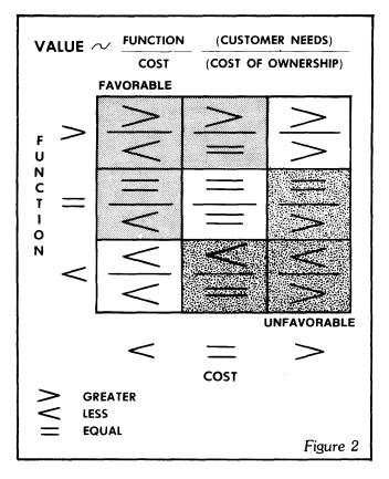
The most desirable relationship is to provide greater functions at less cost. (upper left box)
