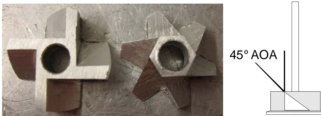
Figure 4.8.11: Pin-wheel Blockage Design and Position on the Valve
