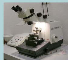
The ultra-microtome is used to cut ultrathin (~60-90 nm) sections of the specimen
