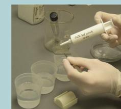
The grids are stained to increase the contrast of the specimen
