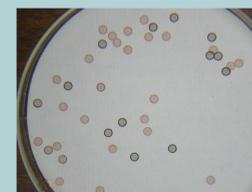
The sections are collected onto fine copper mesh grids
