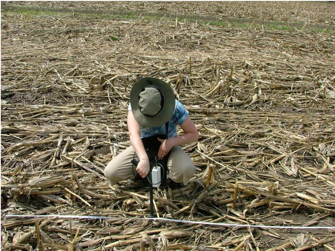
**Figure 9.** Taking surface measurements with the MS2F probe
