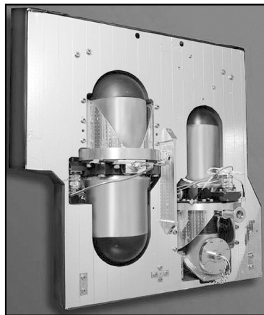
Figure 1. HIRDLS cryocooler mounted into radiator.
