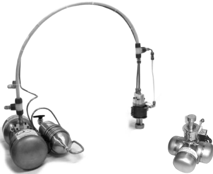
Figure 1. Prototype split acoustic-Stirling system with remote coldhead, using a coldhead rated for 8-10 watts at 77K, driven by an oversized compressor designed for 20-25 watt coldheads, with a 1.3 meter, water-jacketed, 3/8 OD transfer line. The 1/4" OD inertance tube is anchored to the transfer tube with tie-wraps. Our standard 2S102K close-coupled cooler, using the same head with a smaller compressor, is shown for comparison.
