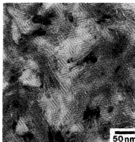
Figure 3: TEM micrographs of the APC composite (top) and a conventionally-processed Nb 48 wt% Ti composite. In the APC composite, the Nb pinning centers are the darker phase, while in the conventional composite, the \alpha -Ti pinning centers appear as the lighter phase.
