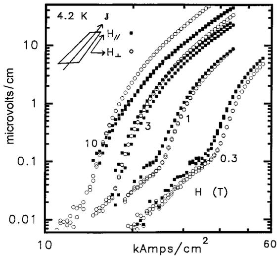
FIG. 2.  $E(J)$  characteristics at 4.2 K for the same tape and field directions as in Fig. 1. The two field directions in the tape plane have an equivalent effect on  $E(J)$ , except at  $H=10$  T and  $E=1 \mu\text{V}/\text{cm}$ . The  $x$  axis is shifted to higher  $J$  than in Fig. 1. The shallower slope at low  $E$  may result from a small component of  $c$ -axis current.
