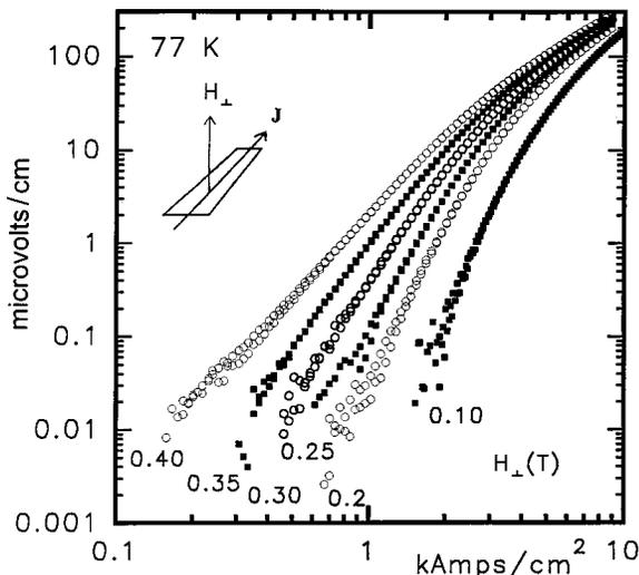
FIG. 3.  $E(J)$  characteristics at 77 K for the same tape as in Figs. 1 and 2, in a field applied orthogonal to the tape plane. The narrower range of orthogonal field displaces the curves over more decades of  $J$  than the wider range of in-plane field in Fig. 1.
