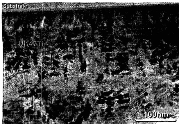
Fig. 4. Transmission electron microscopy image of a 10 nm Nb47Ti / 3 nm Ti multilayer. The sapphire substrate is at the top edge of the photograph. The bright regions are Ti, while the darker gray regions are Nb47Ti. The nearly black regions are grains which strongly diffract the electron beam. The layer structure of the multilayer is evident as horizontal features, while grain boundaries run vertically. Precipitates may also be present, as indicated by the vertical white streaks in the lower left corner.
