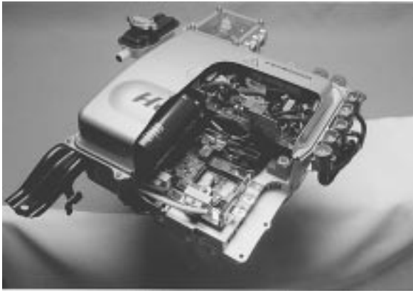
Fig. 15. Cutaway view of Prius power electronics module. (From “Products of Hirose Plant” brochure, courtesy of Toyota Motor Corp.)
