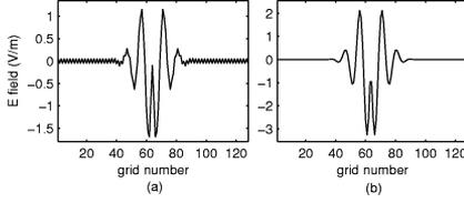
Fig. 1. Spatial distribution of the electric field in a 1-D PSTD grid at an early-time snapshot. A ramped sinusoidal wave is excited in the center of the grid. (a) Single current source is located at  $i_s = 64$ . (b) Two identical current sources are located at  $i_{s1} = 63$  and  $i_{s2} = 64$ .
