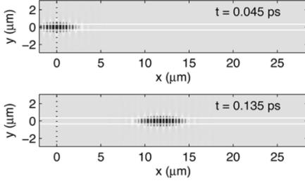
Fig. 3. Visualizations of a pulse propagating in a dielectric slab waveguide. The fundamental waveguide mode has been excited using a twin-source scheme. The white solid and black dotted lines indicate the waveguide geometry and the source location, respectively.
