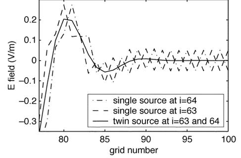
Fig. 2. Performance comparison of single- and twin-source conditions. (Only part of the grid of Fig. 1 is shown here.)
