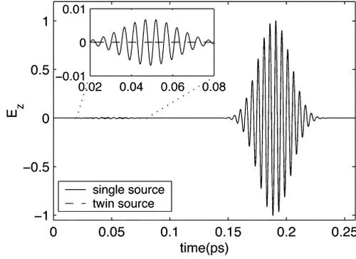
Fig. 4. Temporal evolution of the electric field at an observation point in the waveguide core for two different source conditions.
