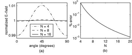
Fig. 5. Anisotropy of a wave radiated by four electric current line sources configured as a quadruplet source. (a) Analytically determined electric field amplitude is plotted at a distance of  $8\lambda$  from the center of the source, as a function of the angle of observation.  $N$  corresponds to the grid sampling density, which dictates the spacing between the current sources. (b) Maximum deviation (percent error) in the field amplitude as a function of grid resolution.
