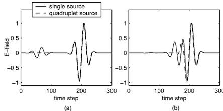
Fig. 7. Temporal evolution of the electric field at the observation points marked by the (a) + and (b) x symbols in Fig. 6 for two different source conditions.
