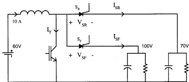
Fig. 5. Schematic of the test circuit used for characterizing active commutation of SCR.
