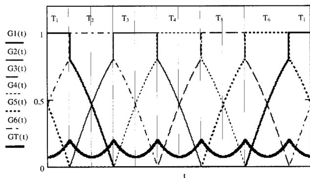
Fig. 10. Modified reference waveforms fed to sine triangle modulator.
