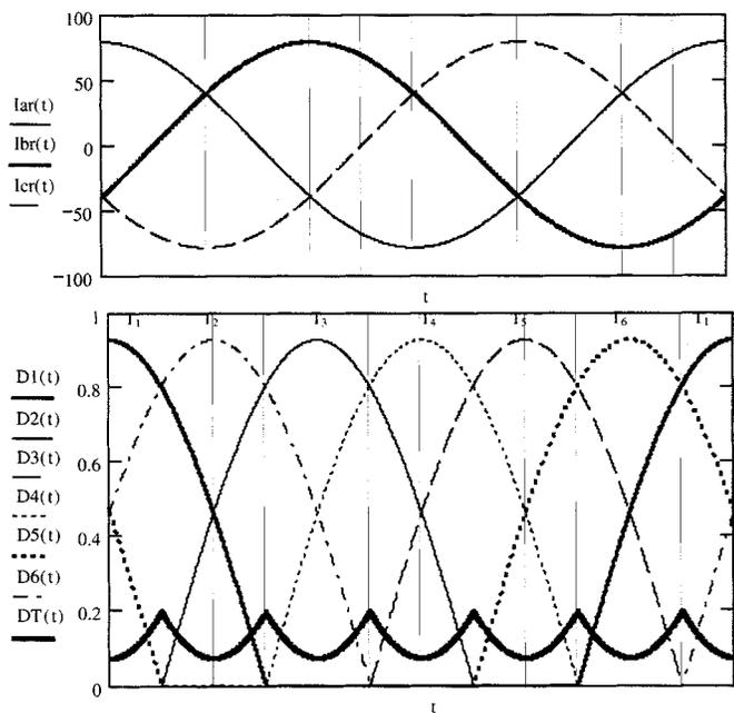
Fig. 9. Waveforms of three phase current references and switch states for the boost inverter.
