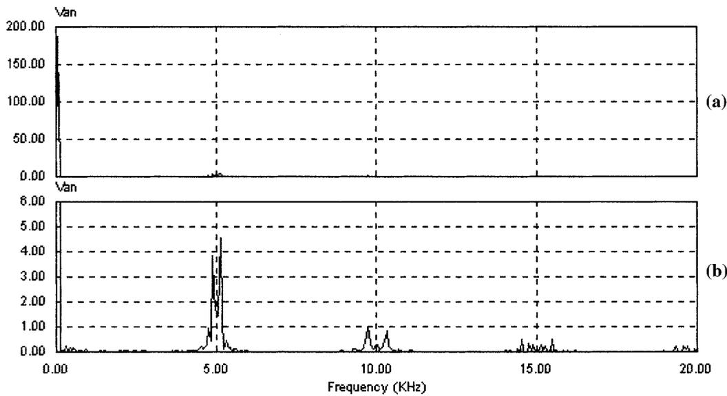
Fig. 14. (a) Spectrum of the  $V_{an}$  with  $D_m = 0.83$  and (b) magnified view.
