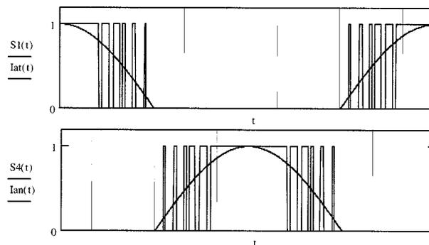
Fig. 11. Gate drive waveforms for  $S_1$  and  $S_4$  and a phase positive and negative reference currents.
