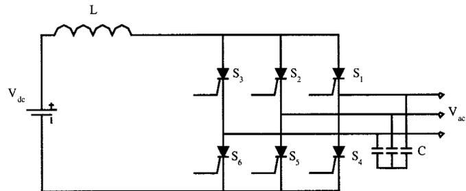
Fig. 1. Schematic of a classical SCR based CSI.
