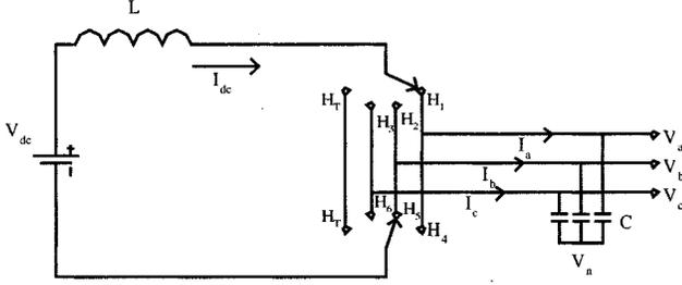
Fig. 8. Ideal switch equivalent circuit of the PWM CSI converter.
