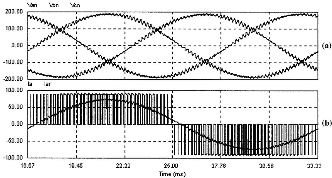
Fig. 13. Inverter output waveforms, operating at  $D_m = 0.83$ : (a) three phase output line-neutral voltages ( $V_{an}$ ,  $V_{bn}$ ,  $V_{cn}$ ) and (b) phase A pole current and sinusoidal load current ( $I_a$ ,  $I_{ar}$ ).
