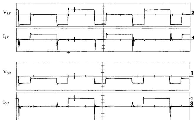
Fig. 7. SCR voltage (50 V/div) and current (5 A/div) waveforms (200  $\mu$ s/div) under active commutation obtained using the experimental test circuit.
