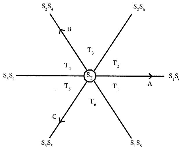
Fig. 12. Phase plane illustration of the switching states of the PWM CSI.
