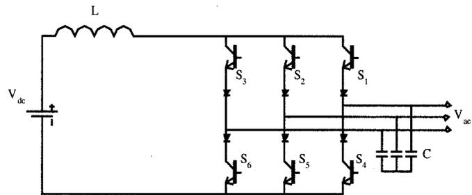
Fig. 2. Schematic of a CSI using IGBTs and series diodes.
