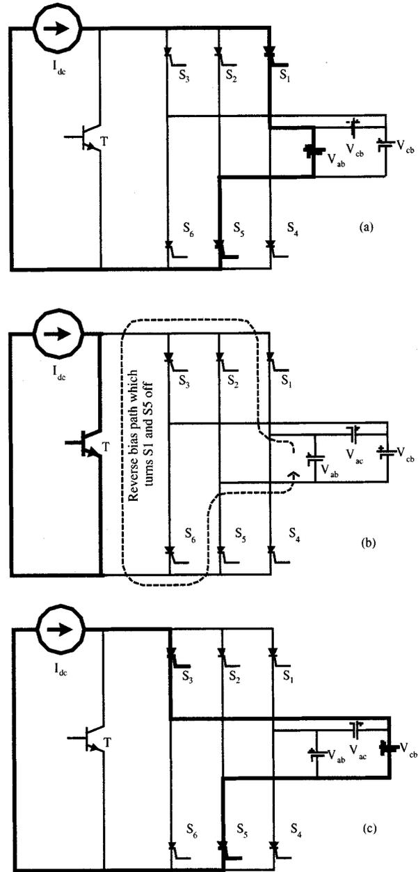
Fig. 4. Schematic of current flow during typical switching states and commutation modes in the proposed converter.
