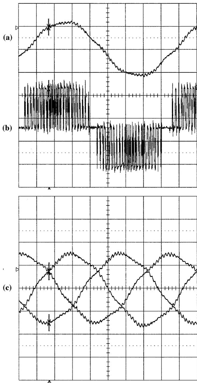
Fig. 15. Waveforms (2 ms/div) of (a) pulse width modulated phase current waveform (5 A/div), (b) load current waveform (2 A/div), and (c) three phase output line-line voltages (50 V/div) from the laboratory prototype actively commutated SCR-PWM inverter switching at 4 kHz.
