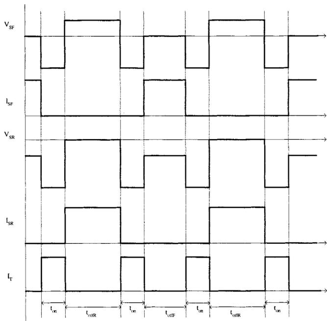
Fig. 6. Ideal test circuit waveforms under different operating intervals during a switching period.
