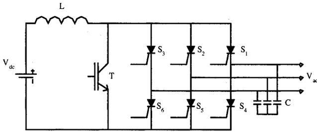
Fig. 3. Schematic of the proposed boost inverter topology.
