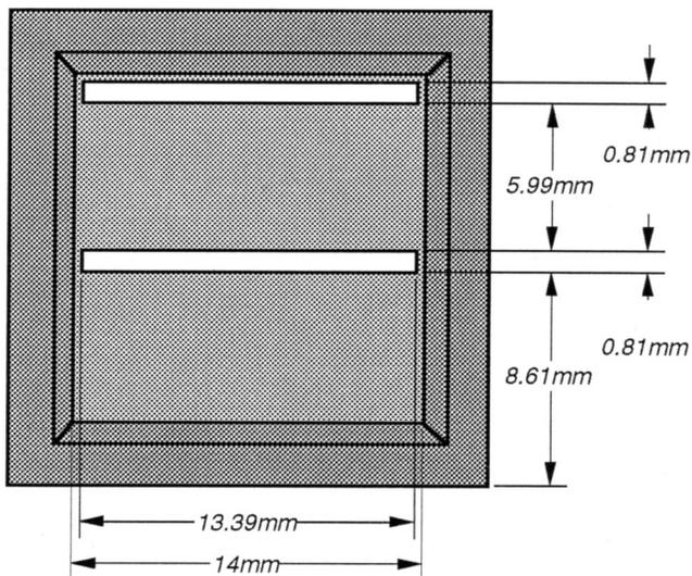
FIG. 4. An example gold mask that allows two exposure windows on a standard  $512 \times 512$  CCD detector.
