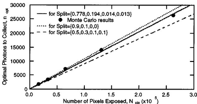
FIG. 3. Optimal number of photons to collect as a function of the number of exposed pixels for different split ratios. The dots represent the results from the Monte Carlo analysis for exposed areas of 512 pixels by 32, 64, 128, 256, and 512 pixels.
