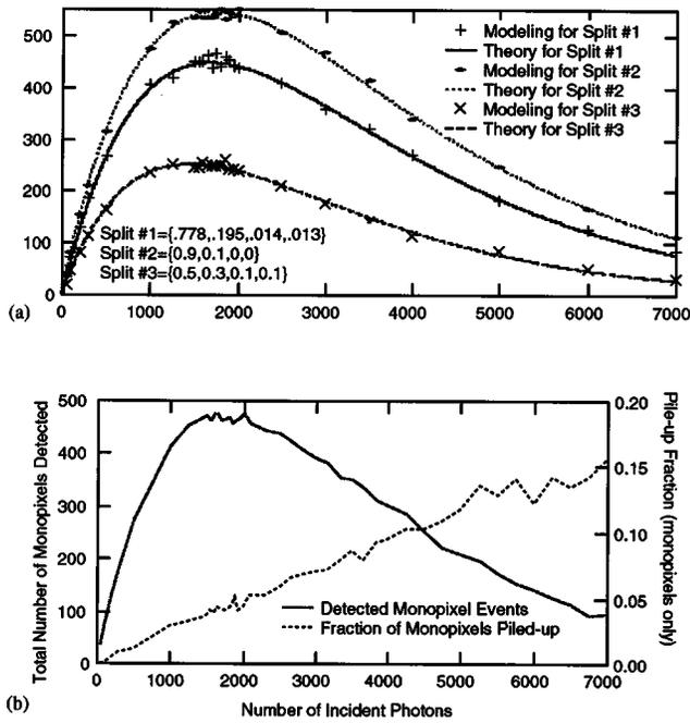
FIG. 2. (a) The number of monopixel photons collected versus number of incident photons for a 200 eV plasma spectrum with 16384 pixels exposed. (b) Total number of monopixel events detected and monopixel pile-up fraction versus number of incident photons.
