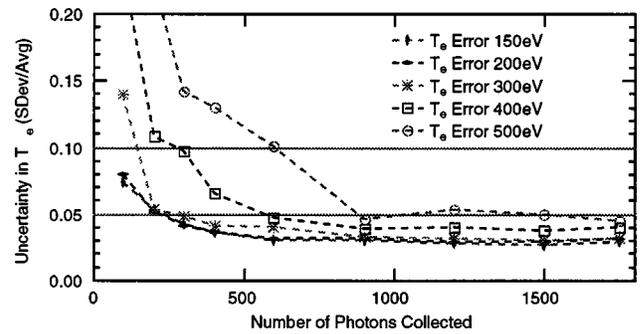
FIG. 5. Error in the temperature fit measurements as a function of number of incident photons for several plasma temperatures, for  $N_{\text{pix}} = 512 \times 32$ .
