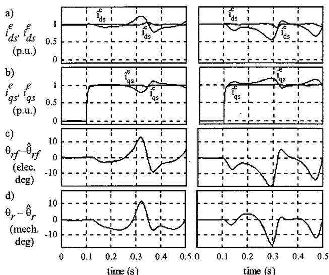
Fig. 8. Simulated field-oriented control and position estimation of a machine with its rotor locked, using a current-model-based flux estimate with (a) no error in its parameters but a 10 electrical degrees error in the decoupling angle of the saturation-induced harmonic and (b) a 20% estimation error in the flux observer rotor resistance and no error in the decoupling angle of the saturation-induced harmonic.
