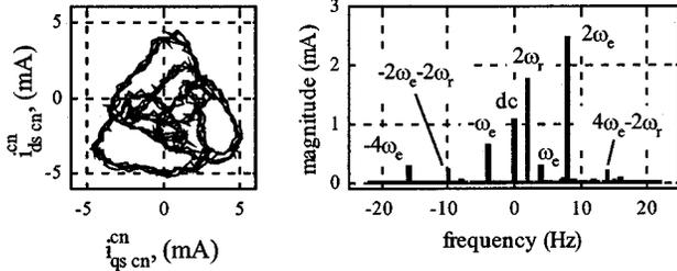
Fig. 1. Negative-sequence carrier-signal current trajectory and frequency spectrum in the negative-sequence carrier-signal reference frame with rated current and rated flux,  $\omega_e = 4$  Hz and  $\omega_r = 1$  Hz, using Motor #1 in Table I. A carrier voltage of  $V_c = 7$  V and frequency of  $\omega_c = 535$  Hz were used.
