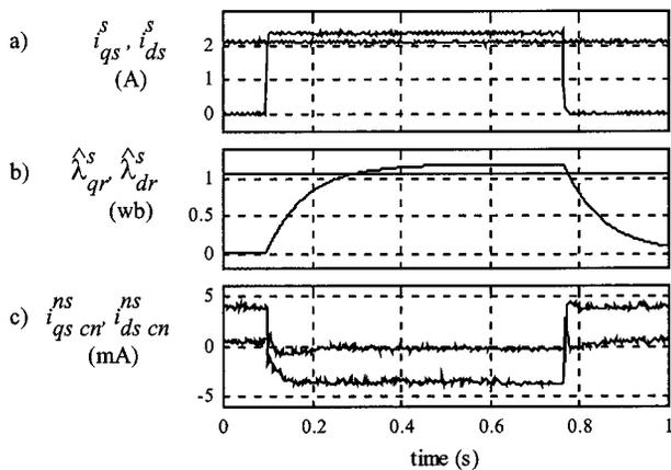
Fig. 11. Experimental results showing (a) dynamic response of the  $q$ -axis current in a stationary reference frame, with the  $d$ -axis current kept constant, and the rotor locked, (b) estimated rotor flux in a stationary reference frame, and (c)  $q$  and  $d$  components of the negative carrier-signal current during the transient in the fundamental current, with the fundamental current decoupled by means of a fundamental current observer.
