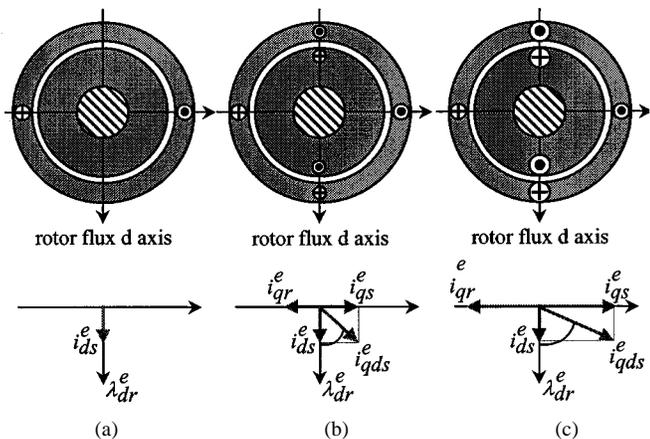
Fig. 4. Schematic representation of the relative position between the rotor flux and the stator current for the case of rated flux and three different levels of load, shown in a rotor-flux reference frame for a two-pole machine. (a) Rated flux, no load. (b) Rated flux, light load. (c) Rated flux, full load.
