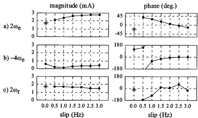
Fig. 3. Magnitude and phase, relative to the fundamental current, of the most significant negative sequence harmonics as a function of the slip frequency, for Motor #2 in Table I, operated under the same condition stated in Fig. 2.
