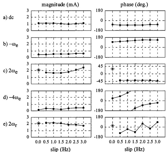
Fig. 2. Magnitude and phase, relative to the fundamental current, of the most significant negative-sequence harmonics as a function of the slip frequency for Motor #1 in Table I. The motor was operated at rated rotor flux with the  $q$ -axis current varied proportional to the slip. A constant fundamental excitation frequency  $\omega_p = 4$  Hz was used, the rotor frequency was varied from  $\omega_r = 4$  Hz (slip = 0 Hz) to 1 Hz (slip = 3 Hz). A carrier frequency of 535 Hz was used.
