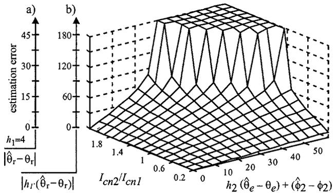
Fig. 6. Maximum rotor position estimation error in mechanical degrees as a function of the relative magnitude of the negative-sequence carrier-signal current induced by the rotor saliency and the secondary saliency,  $I_{cn1}$  and  $I_{cn2}$ , respectively, and the estimation error in the secondary saliency decoupling angle, for the case of a machine with  $p = 4$  and  $h_1 = 4$ .
