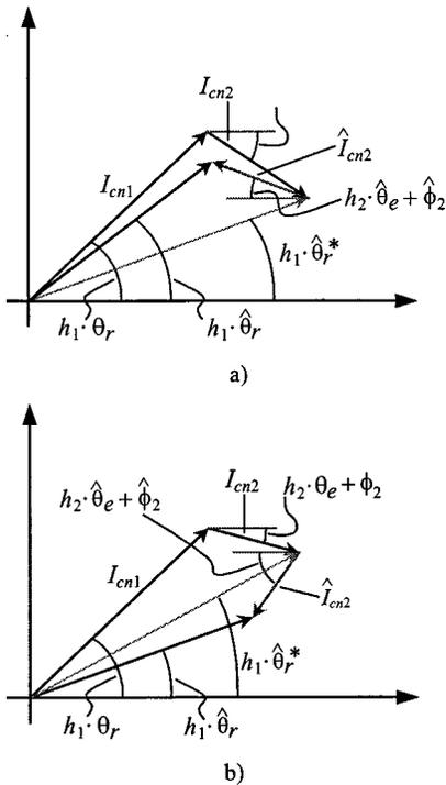
Fig. 5. Estimation error resulting from inexact decoupling of a secondary harmonic. (a) Secondary harmonic with a small error in the decoupling angle. (b) Secondary harmonic with a large error in the decoupling angle.
