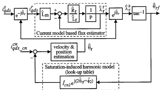
Fig. 7. Rotor flux angle estimation using a current-model-based flux estimator (shown in a rotor position synchronous reference frame) and decoupling of a saturation-induced harmonic dependent on the rotor flux position. The machine has a rotor-position-dependent saliency and a saturation-induced saliency, both with a harmonic order  $h$  equal to the pole number.
