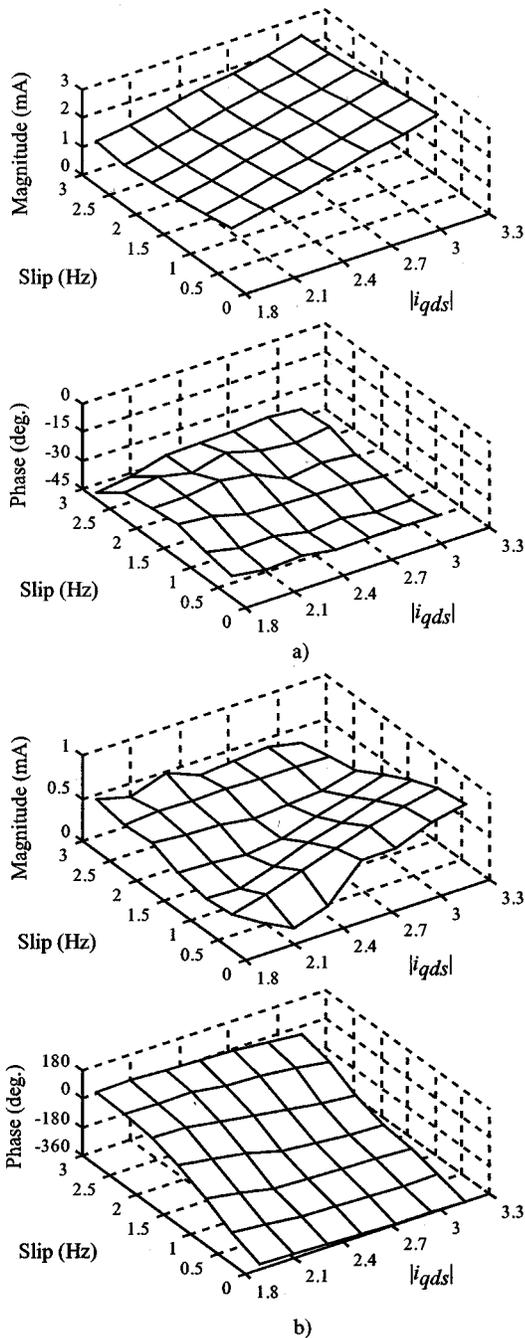
Fig. 9. Magnitude and phase (relative to the fundamental current) of the (a)  $2\omega_e$  and (b)  $-4\omega_e$  fundamental-excitation-dependent negative-sequence harmonics as a function of the slip frequency and fundamental current level, for Motor #1 in Table I. A constant fundamental excitation frequency  $\omega_e = 4$  Hz was used, with the rotor speed varied according to the slip shown in the figure. A carrier frequency of 535 Hz was used.
