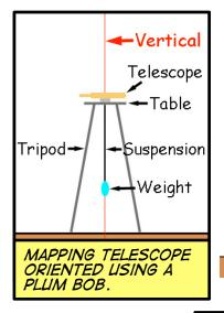
PLUM BOBS ARE USED TO FIND VERTICAL-A WAY TO MAKE SURE YOUR INSTRUMENT IS HORIZONTAL. BOUGUER WAS AWARE THAT THE EXTRA MASS OF THE ANDES WOULD ATTRACT THE WEIGHT AND SO HE MADE A CORRECTION FOR THIS EFFECT.
