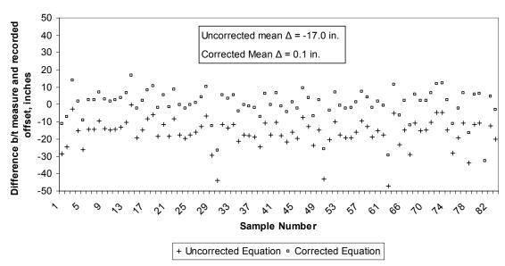
Figure 1-7- Wheel wander offset calibration data.
