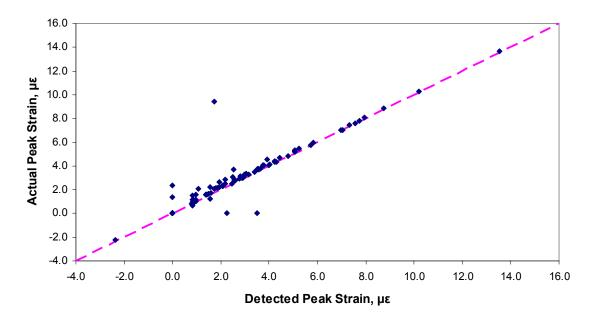
Figure 2-7 - Actual versus detected peak tensile strains.
