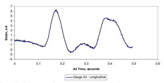
Figure 1-10 - Strain response from quad axle dump with pusher axle up.
