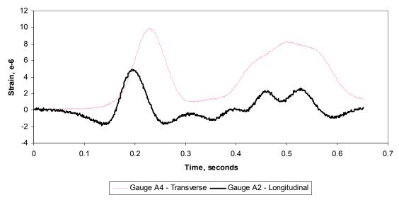
Figure 1-9 - Strain response from quad-axle dump truck.
