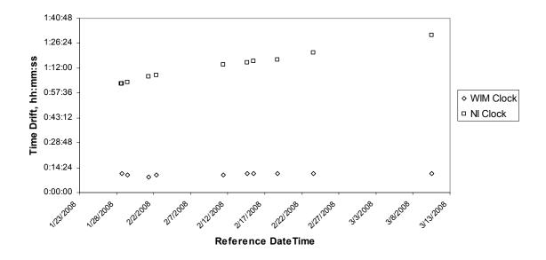
Figure 1-12 - Time drift for WIM and NI systems.
