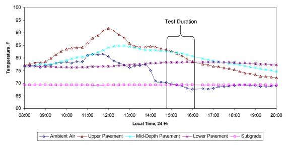
Figure 1-6 - Pavement temperatures during testing.
