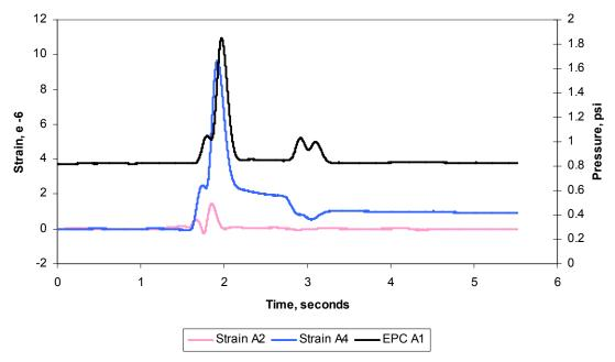
Figure 1-2 - Strain and pressure signals from test vehicle.
