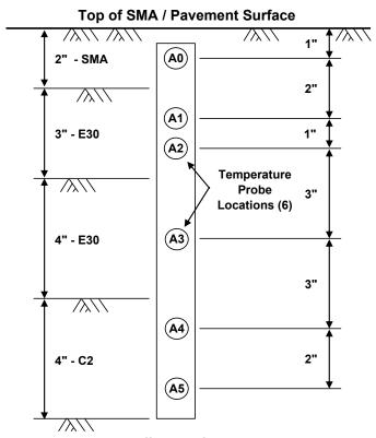
Figure 1-1 - Pavement temperature gradient probe.
