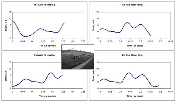
Figure 2-4 - Quad axle strain signals.
