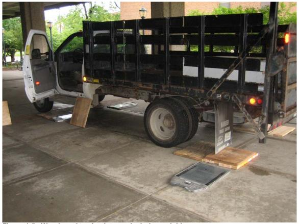
Figure 1-5 - Wood used to simulate grade during weighing.
