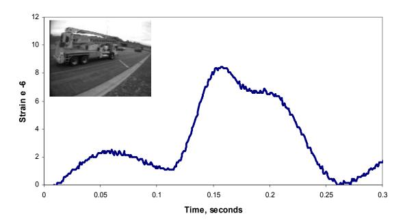
Figure 2-5 - Tandem axle strain signal.
