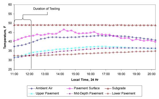
Figure 1-11 - Pavement temperatures during testing.
