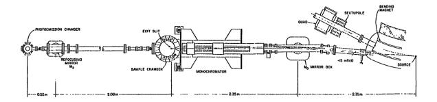
Fig. 2 A typical beamline on Aladdin showing a dipole bending magnet, a mirror box accepting 15 mr of beam, a grazing incidence monochromator and two alternate sample chambers.
