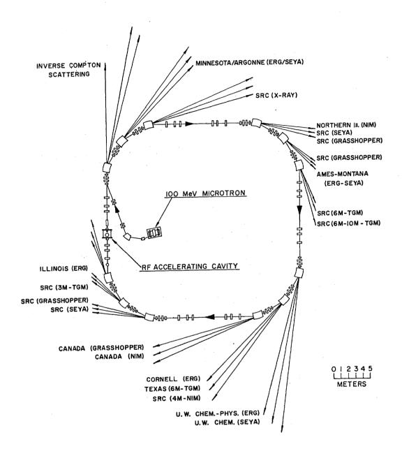
Fig. 1 Schematic of the Aladdin 1 GeV electron storage ring showing the microtron injector, the transport line, the storage ring, and the RF cavity. The twenty-one beamlines are identified according to principal investigators or the facility.
