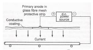
**Figure 17:** Conductive coating ICCP (6)
