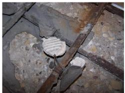
**Figure 306:** Close-up of EA-A w/A-C(1) exposed rebar after 6-months
