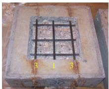
**Figure 341:** Condition of EM(2) exposed rebar after 3-months
