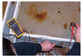
Figure 100: Half-cell potential measurement
