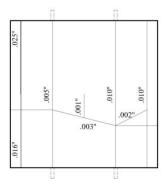
**Figure 284:** Crack-mapping of EA-A(1) after 3-months
