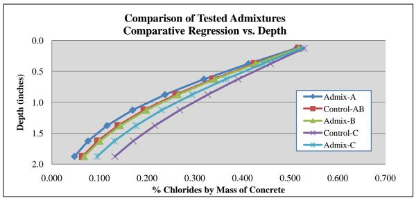
**Figure 364:** Comparative regression analysis of tested admixtures
