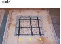
**Figure 245:** Condition of Control(2) exposed rebar after 3-months
