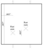
**Figure 140:** Crack-mapping of EA-A w/A-C(1) after 6-months
