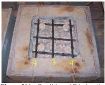
**Figure 301:** Condition of EA-A w/A-C(1) exposed rebar after 3-months
