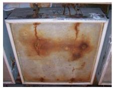
Figure 259: Condition of TSZ w/EP-C(2) after 3-months
