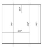
**Figure 316:** Crack-mapping of EA-B(1) after 3-months
