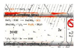
Figure 11: Corrosion cell in concrete (12)
