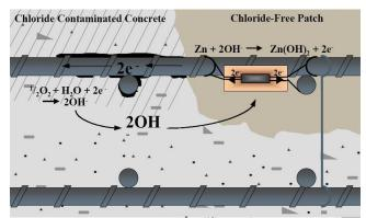
Figure 18: Discrete anode GCP (12)
