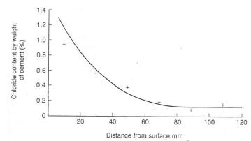
Figure 8: Profile of chloride content vs. depth (6)
