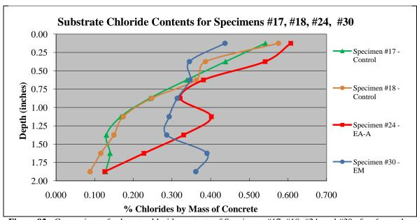
Figure 92: Comparison of substrate chloride contents of Specimens #17, #18, #24, and #30 after 6-months
