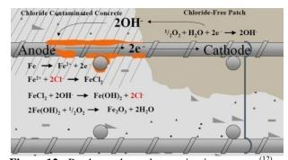
Figure 12: Patch-accelerated corrosion in concrete (12)
