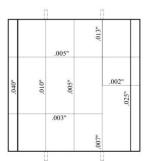
**Figure 180:** Crack-mapping of EA-B(2) after 6-months
