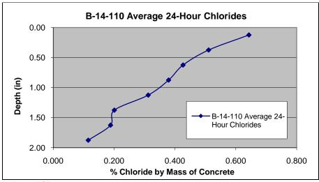
Figure 358: Average Chloride Content of Locations for Bridge B-14-110
