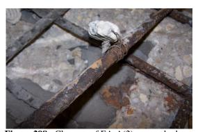
**Figure 298:** Close-up of EA-A(2) exposed rebar after 6-months
