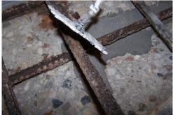
**Figure 258:** Close-up of TSZ w/EP-C(1) exposed rebar after 6-months
