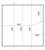
**Figure 260:** Crack-mapping of TSZ w/EP-C(2) after 3-months
