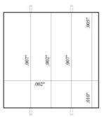
**Figure 324:** Crack-mapping of EA-B(2) after 3-months
