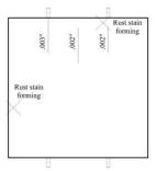
**Figure 202:** Crack-mapping of A-C after 3-months
