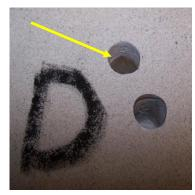
**Figure 96:** Discoloration in EM (Location D) of Specimen #30
