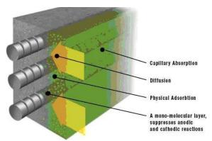
Figure 13: Surface applied corrosion inhibitor (36)
