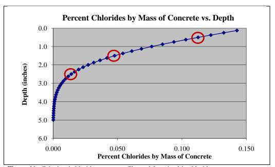
Figure 46: Calculated chloride content profile used for mixed-in chlorides
