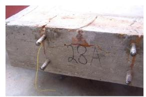
**Figure 65:** Existing cracks on the sides of the CoC specimens
