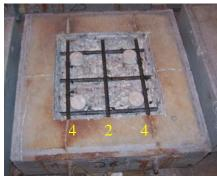
**Figure 309:** Condition of EA-A w/A-C(2) exposed rebar after 3-months
