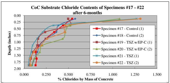
Figure 91: CoC substrate chloride contents of Specimens #17 through #22 after 6-months
