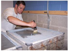
**Figure 36:** Application of humectant activator
