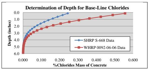
Figure 360: Calculated depth at which chlorides would not be present
