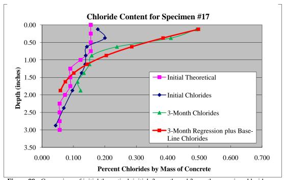
**Figure 90:** Comparison of initial theoretical, initial, 3-month, and 3-month regression chlorides for Specimen #17
