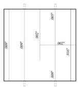
**Figure 332:** Crack-mapping of EM(1) after 3-months
