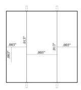
**Figure 308:** Crack-mapping of EA-A w/A-C(2) after 3-months
