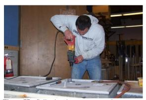
Figure 77: Collecting the concrete powders
