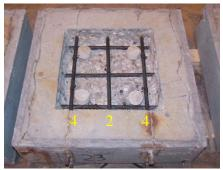
**Figure 285:** Condition of EA-A(1) exposed rebar after 3-months
