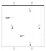
**Figure 236:** Crack-mapping of Control(1) after 3-months
