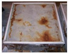
**Figure 243:** Condition of Control(2) after 3-months
