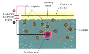
**Figure 21:** Electrochemical chloride extraction (12)
