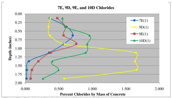
Figure 82: Chloride profiles for Locations 7E(1), 9D(1), 9E(1), and 10D(1)
