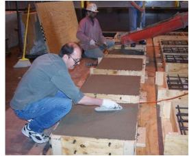
Figure 48: Finishing the CoP specimens
