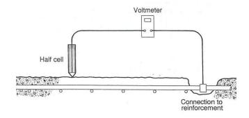
**Figure 10:** Half-cell potential test <sup>(6)</sup>
