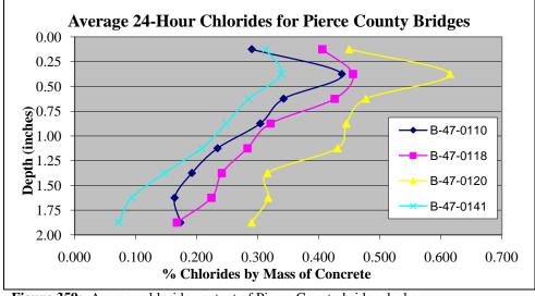
Figure 359: Average chloride content of Pierce County bridge decks
