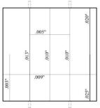
**Figure 172:** Crack-mapping of EA-B(1) after 6-months
