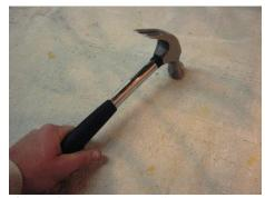
Figure 6: Hammer sounding
