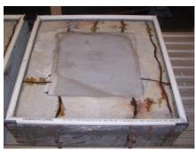
**Figure 327:** Condition of EA-B(2) after patch repairs
