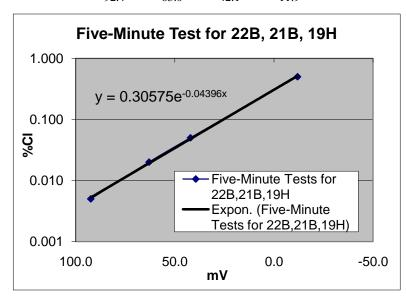
Calibration values based on difference of 0.050% Cl checks.
