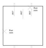
**Figure 204:** Crack-mapping of A-C after 6-months
