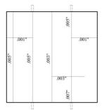
**Figure 218:** Crack-mapping of Control(1) after 3-months
