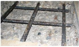
**Figure 286:** Close-up of EA-A(1) exposed rebar after 3-months
