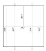
**Figure 244:** Crack-mapping of Control(2) after 3-months
