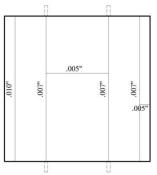
**Figure 292:** Crack-mapping of EA-A(2) after 3-months
