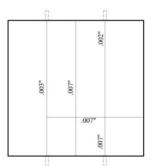
**Figure 108:** Crack-Mapping of TSZ(1) after 6-months
