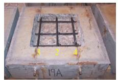
**Figure 253:** Condition of TSZ w/EP-C(1) exposed rebar after 3-months
