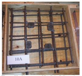
Figure 32: Placement of EA-B in CoP specimens
