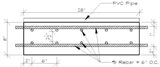
Figure 42: Cross section of concrete specimen
