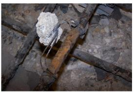
**Figure 322:** Close-up of EA-B(1) exposed rebar after 6-months
