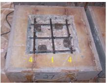
**Figure 317:** Condition of EA-B(1) exposed rebar after 3-months
