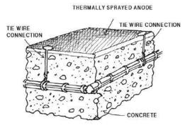
**Figure 19:** Thermal sprayed GCP <sup>(59)</sup>
