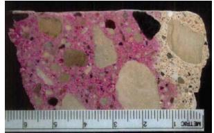
**Figure 9:** Concrete sample displaying depth of carbonation
