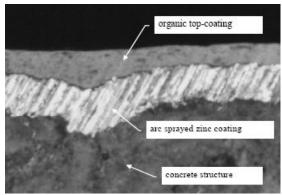
**Figure 20:** Application of a top-coating to thermal sprayed zinc <sup>(60)</sup>
