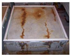
**Figure 251:** Condition of TSZ w/EP-C(1) after 3-months
