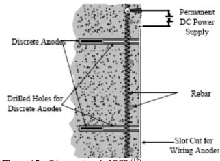
Figure 15: Discrete Anode ICCP
