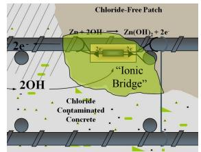
**Figure 41:** Low resistivity ionic bridge between anode and substrate concrete (113)
