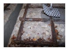
**Figure 274:** Close-up of TSZ(1) exposed rebar after 6-months
