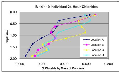
Figure 357: Individual Chloride Content of Locations of Bridge B-14-110
