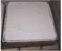
**Figure 264:** Condition of TSZ w/EP-C(2) after 6-months
