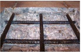
**Figure 310:** Close-up of EA-A w/A-C(2) exposed rebar after 3-months
