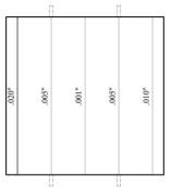
**Figure 276:** Crack-mapping of TSZ(2) after 3-months
