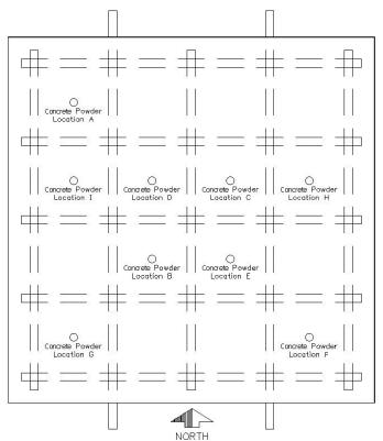
Figure 56: Location of laboratory concrete powders
