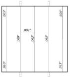
**Figure 156:** Crack-mapping of EA-A(1) after 6-months
