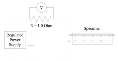
Figure 51: Corrosion cell for laboratory specimens
