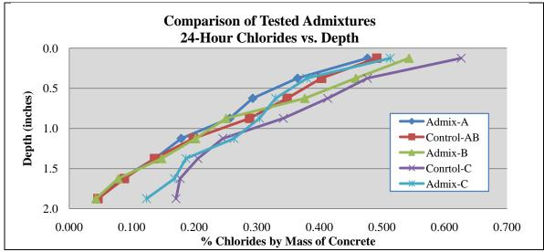
Figure 363: Comparison of chloride contents of tested admixtures
