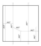
**Figure 268:** Crack-mapping of TSZ(1) after 3-months
