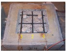
**Figure 293:** Condition of EA-A(2) exposed rebar after 3-months
