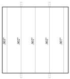
**Figure 226:** Crack-mapping of Control(2) after 3-months
