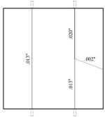
**Figure 340:** Crack-mapping of EM(2) after 3-months
