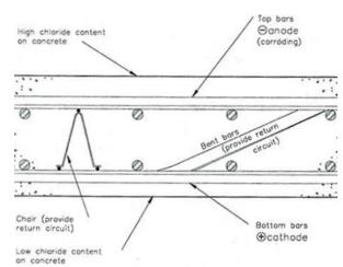
Figure 3: Corrosion "macrocell" (7)
